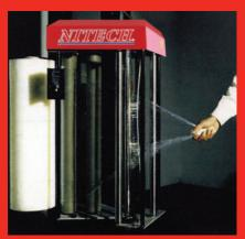
Quick threading feature Pull-out cage enables film to be pulled across rollers easily.
