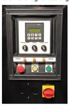
LCD with menu and instructions for program and sequence selection. Touch key pad to select and store program options. Status lights indicate power, ready, and tension. Knobs to adjust turntable speed, film tension and elevator speed. Industrial push button controls for stop, control on/pause, start/resume and turntable jog.
