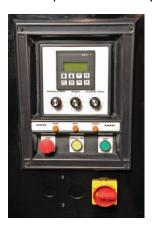
LCD with menu and instructions for program and sequence selection. Touch key pad to select and store program options. Status lights indicate power, ready, and tension. Knobs to adjust turntable speed, film tension and elevator speed. Industrial push button controls for stop, control on/pause, start/resume and turntable jog.
