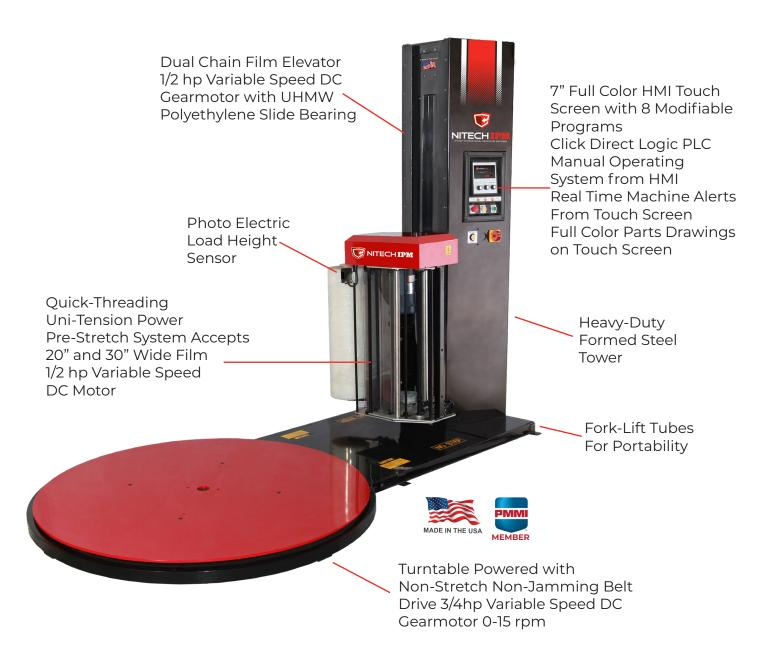
60" Round Turntable, 3" Table Height 6,000 lbs. Capacity Operates on 115 Volts, 50/60HZ 20ft. Power Cord Low Maintenance 4 Year Parts Warranty 5 Year Structural Warranty Optional Loading Ramp and Scale Availble
