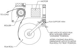
The fixed ratio UTS power pre-stretch system is available with constant tension spring dancer, and has incorporated a quick-threading cage. Simply open the cage, pull the film across the front of the unit and close the cage. The film is automatically threaded around the urethane stretch rollers, idler rollers and dancer. A plexiglass safety shield protects the operator from rotating rollers. Stretch ratios of 200%, 225%, 250% and 300% are available with the UTS film delivery.
